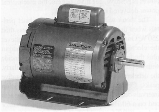
Figure 18.15 Single-phase capacitor-start motor supported in a resilient-mount cradle to reduce the vibration and noise transmitted to the mounting surface. Motor rated at 1/3 hp, 1725 r/min, 230 V, 60 Hz has a full-load current of 3.0 A, efficiency of 60 percent, and power factor of 60 percent. Other characteristics: no-load current: 2.6 A; locked-rotor current: 13 A; locked rotor torque: 3.6 pu; breakdown torque: 3.0 pu; service factor: 1.35; total weight: 10 kg; overall length including shaft: 278 mm; overall height: 232 mm. (Courtesy of Baldor Electric Company)
